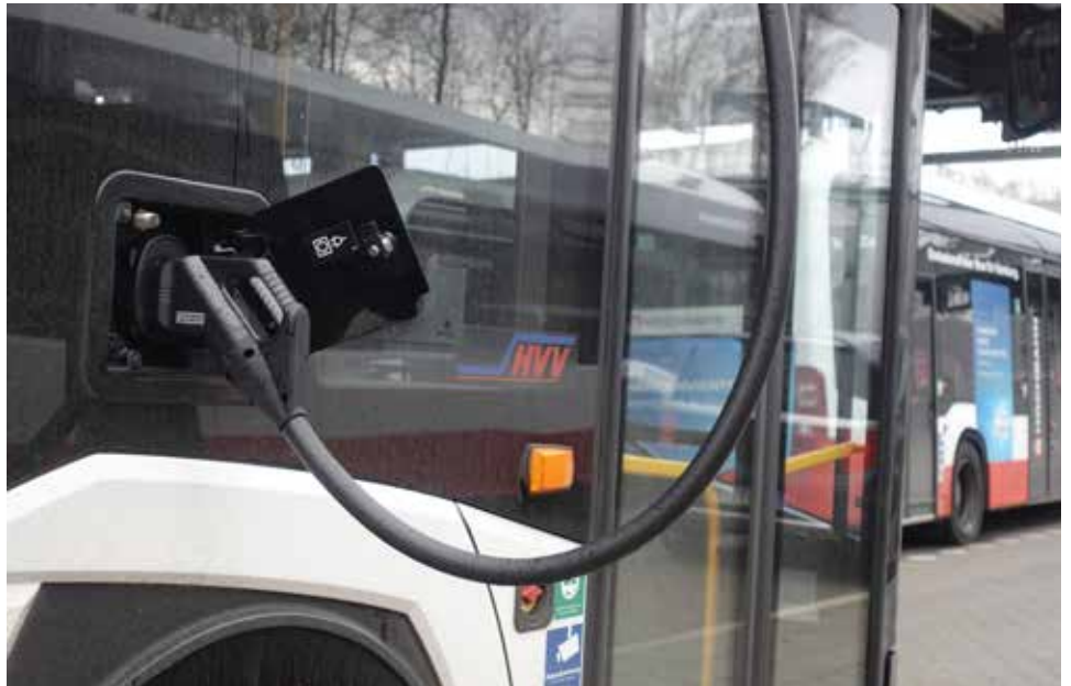
At Hamburger Hochbahn AG, the VDV 463 interface was developed in a pilot project.
