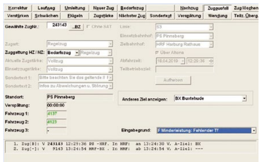
As an example: The figure shows an offline dialogue in which the itinerary of a train is to be shortened using a dispatching measure. The dispatcher opens the dialogue and edits the measure. The measure is not implemented until the dialogue has been closed. If the train has already left the station at which the train formation change is to be carried out, the dispatcher only sees this after closing the dialogue.
