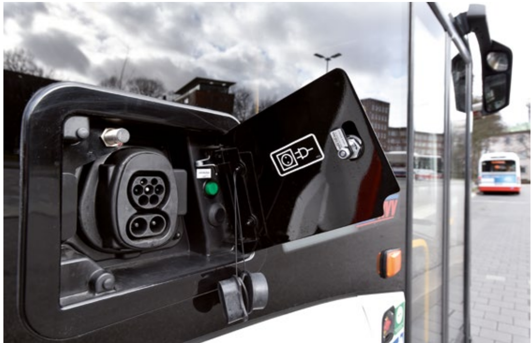
The fact is: Plug-in charging socket of a Solaris bus.
